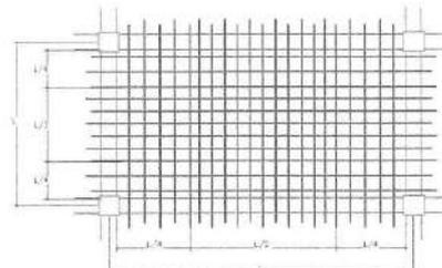
TYPICAL CONCRETE SLAB PLAN & DETAIL SHOWING BOT. BARS
