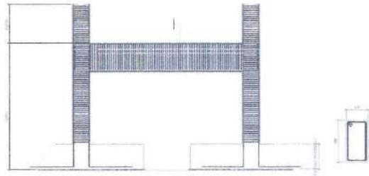
TYPICAL FOOTING TIE BEAM DETAIL
