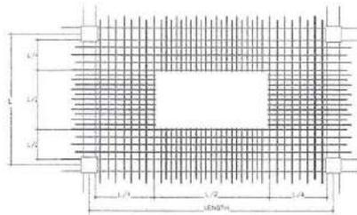
TYPICAL CONCRETE SLAB PLAN & DETAIL SHOWING TOP BARS
